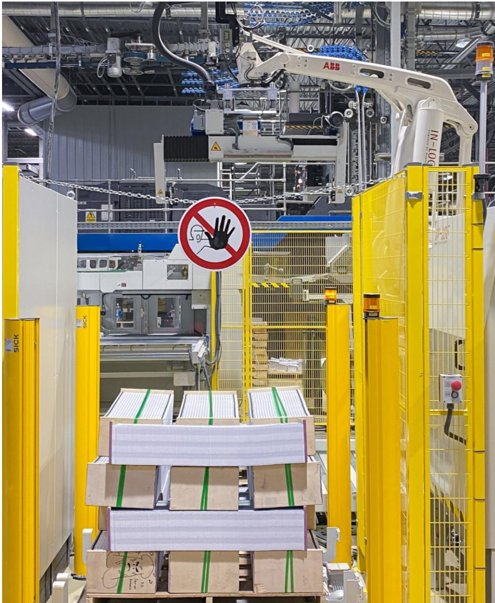
▲ The robot can place the logs side by side but also "criss-cross"
