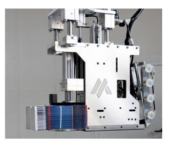
▲ Handles loose, strapped, and film-wrapped bundles, up to 350 bundles/hour. The single gripper is just one of several ways to configure the ERIC mini-robot. The optional rear-mounted slip sheet gripper allows slip sheets to be placed onto defined layers.
