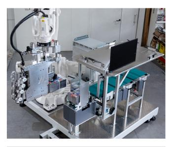
▲ All-in-one and mobile! ERIC is built on a frame that integrates the robot arm, the infeed and an optional slip sheet table. Two operators can easily move the mini-robot between different lines and use it where it makes the most sense.
